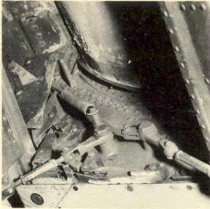
Bent latch handle (left above) holds over-center plunger linkage in half-released position. Proper
