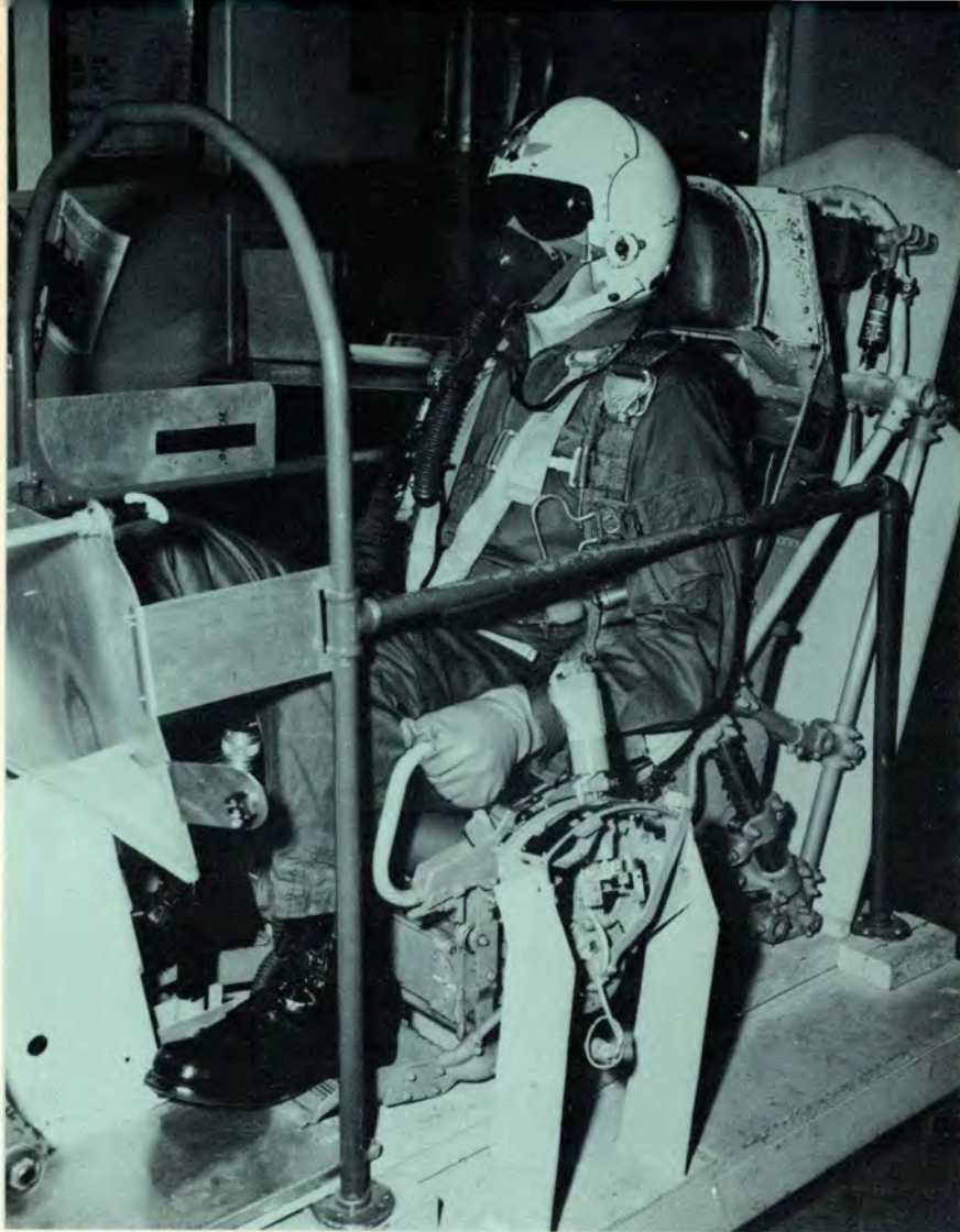
Thumper drags pilot lying on mattress with series of jerks that simulates dragging by parachute canopy.
