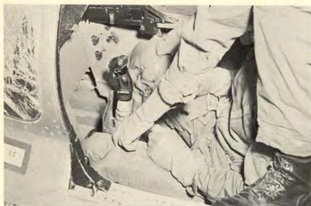
Salvaged F-100 fuselage provides egress and rescue training. Fireman wearing protective gear practices opening canopy. Pilot removal technique calls
