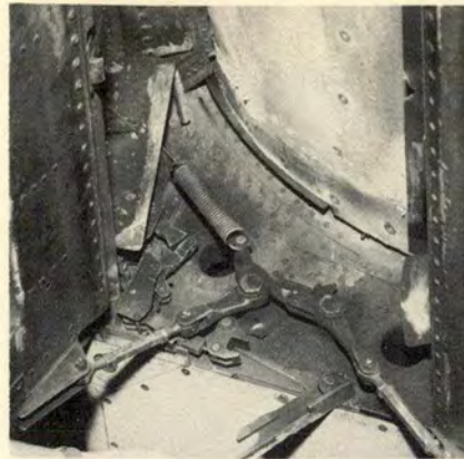
Bent latch handle (left above) holds over-center plunger linkage in half-released position. Proper
